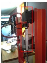
17) Holding a **stopwatch**, open the **pressure regulator** to pressurize the system and apply 193 lbs for the first loading (the plunger assembly weighs 7 pounds). Monitor the force and displacement displays; they should be increasing accordingly. Once 193 lbs is reached\*, start stopwatch and record displacements at the time intervals described in the data sheet. You should note a signal on
