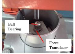
13) Power on both the load and the **displacement indicator boxes** (use the switch on the power strip on the back of the computer shelf). Zero the load indicator ('tare' button). Power on the oscilloscope, use preset settings (if these are not correct press 'save/recall setup', 'recall saved setup', 'recall setup2 user', 'clear menu').
