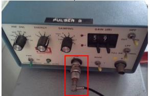
Connect the lower transducer wire to the left port in the
