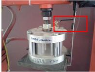
11) Move the assembly to the orange **test frame** and connect the upper transducer wire to the **Pulser box** in the "T/R" transmit receiver port.
