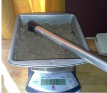
6) Using the spoon, transfer approximately 160 g of material to the **sample cylinder**. Try to distribute the material evenly across the bottom of the cylinder. Tamp the material 25 times. To keep the sample as level as possible while tamping, move the tamper around
